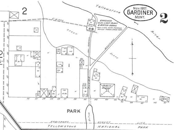
Detail of 1907 Sanborn map showing location of feeder ditch and Gardiner Electric Light and Water Company pump and power house location.
